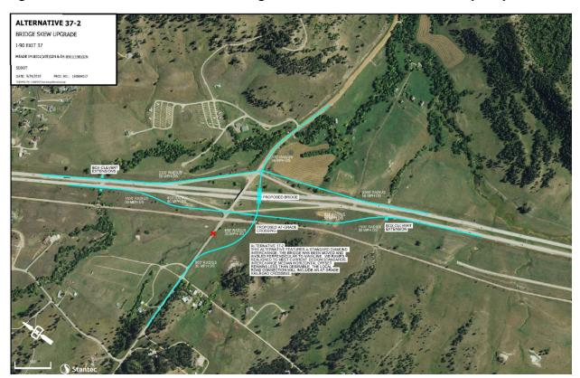
Figure ES-1. I-90 and Exit 37 Interchange Modification Build Alternative (37-2)
