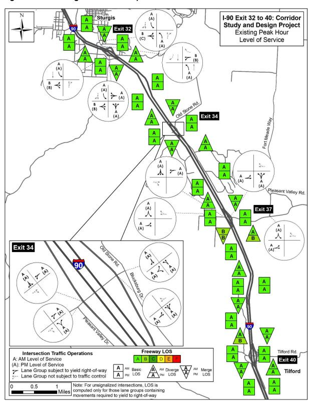
Figure 3-8 Existing Peak Hour Delay and LOS
