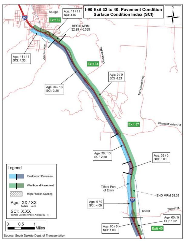
Figure 4-1 Pavement Condition Surface Condition Index
