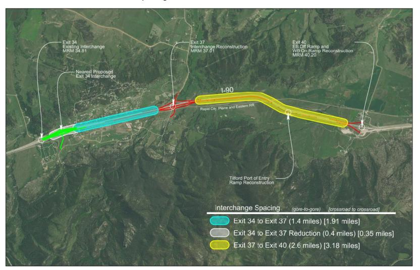
**ALTERNATIVE 40-1** STANDARD DIAMOND UPGRADE I-90 EXIT 40 MEADE IM 0901(195)32N & IM 0901(198)32N SDDOT PROJ. NO.: 193804017 DATE: 9/24/2018 ALTERNATIVE 40-1 WB ON-RAMP AND EB OFF-RAMP ALIGNED TO MEET CURRENT DESIGN STANDARDS. Stantec
